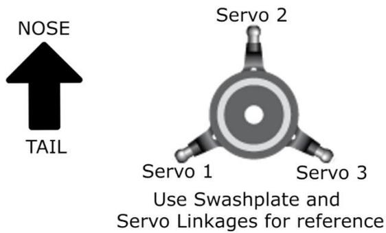
Using the Swashplate for reference. Follow the diagram here to trace the control linkage from the corresponding Swashplate arm down to the servo. A helpful tip, if you are having trouble, is to plug in a single servo into any of the 3 Servo Ports, power on the model, and see which one centers and moves. Using this procedure will help determine where each servo is located in reference to the swashplate diagram.
