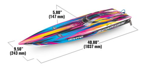
MODEL 57076-4: Fully assembled, Ready-To-Race®, TQi™ 2.4GHz radio system, Traxxas Stability Management®, Velineon® 540XL Brushless Motor, VXL-6s Marine ESC, and factory-applied graphics.
